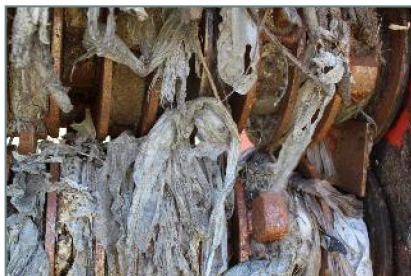
Compostable bags and paper cups stuck in the grinding equipment at the LRCRC.
